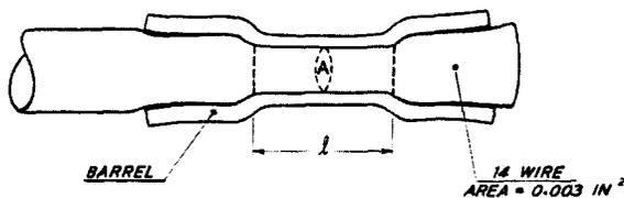
$l_e \approx 0.1$  INCH = EFFECTIVE LENGTH OF CRIMPED WIRE
